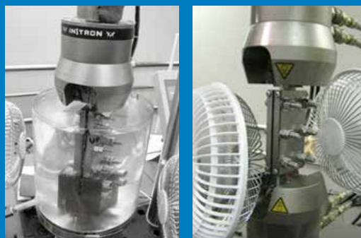
In-Water and In-Air Test Configurations
